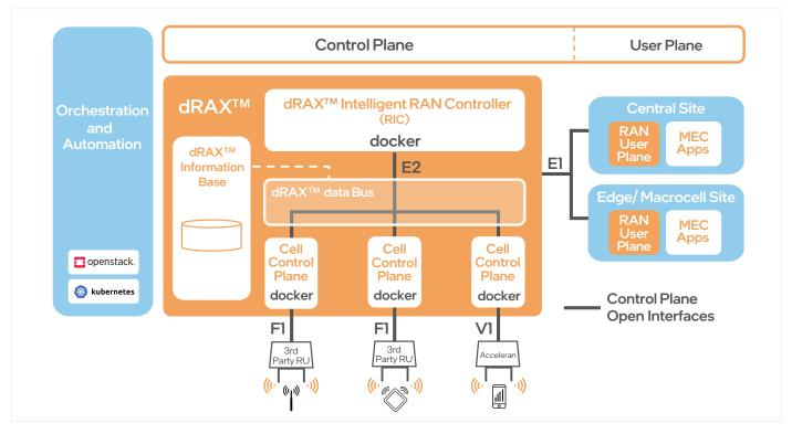
Figure 2. Accelleran dRAX block diagram.
