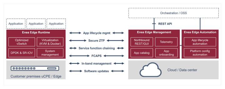
Figure 4. A schematic view of Enea Edge in a typical deployment.
